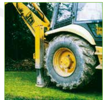
Grassrings can withstand loadings in excess of highway maximums
